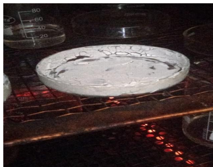
Figure 3: Drying of the ZnO precipitate to obtain ZnO nanoparticle powder
